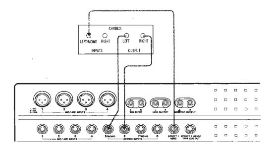
Mono returns: A special feature of the STEREO INPUTS allows continuously variable control between left and right if desired: a mono effect connected to 5/MONO (or 7/MONO) will go to "5-6" (or "7-8") LEVEL control if nothing is plugged into its companion jack (even-numbered).
