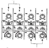
These mixer channels are being sent to the RIGHT, for recording on either Track 2 or Track 4.
