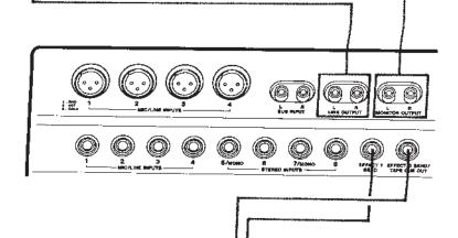
**EFFECT 1 SEND**: For sending post-fader signals to effects devices. The returns are plugged into the STEREO INPUTS.
