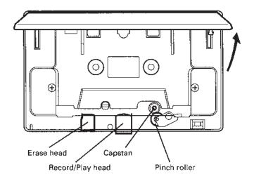
Using a good head cleaning fluid and a cotton swab, clean the heads and tape guides until the swab comes off clean. Wipe off any excess cleaning fluid with a dry swab.
